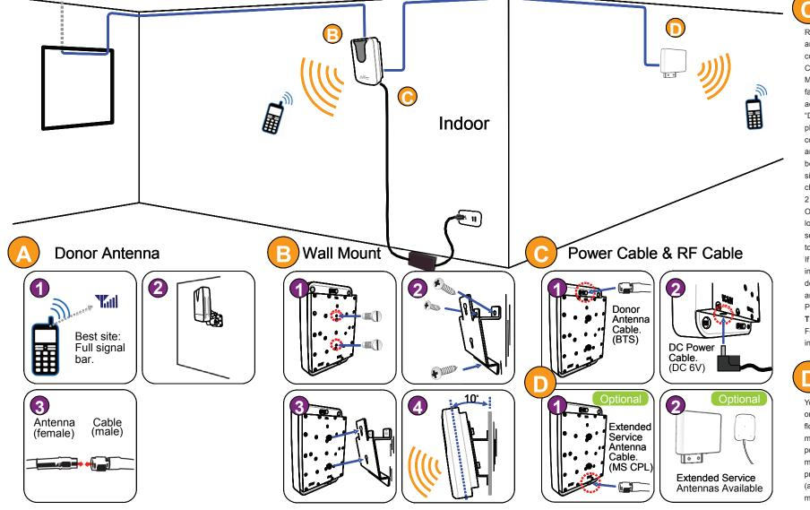
Route the cable between the donor antenna and the repeater unit. Connect the cable to the connector marked BTS on the repeater. Connect the other end to the donor antenna. Make sure that all of the connections are tightly fastened. Connect the power cable of the adaptor to the main unit where indicated "DC6V", and plug the adaptor into the power
